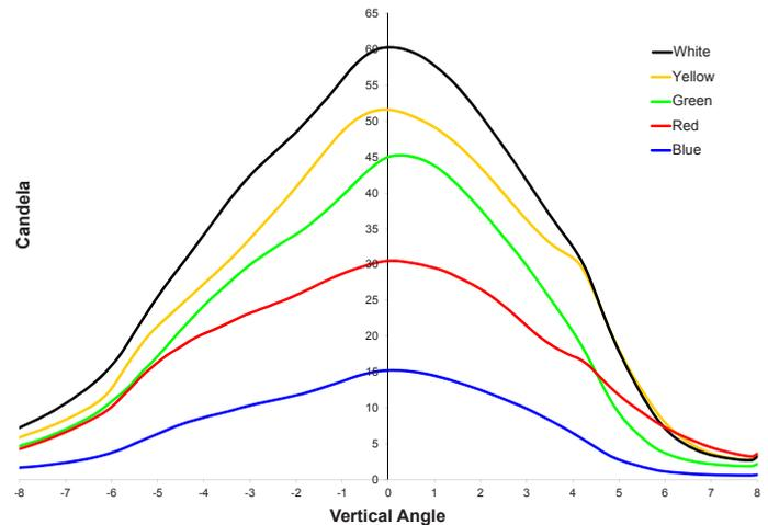
Note: Peak IALA intensity dependent on location. Plot based on equatorial location of 12-hour night duration and 21% duty cycle flash code.
